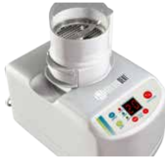
FIGURE 23: The Smart Dentin Grinder (GoldenDent) is used to grind the patient's roots into an autogenous graft particulate. It is a self contained unit and consists of a motor and a disposable chamber, as well as a cleanser and saline wash vials.
